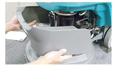
6. Remove existing pedal latch bracket from machine frame and discard. Install new latch bracket.
